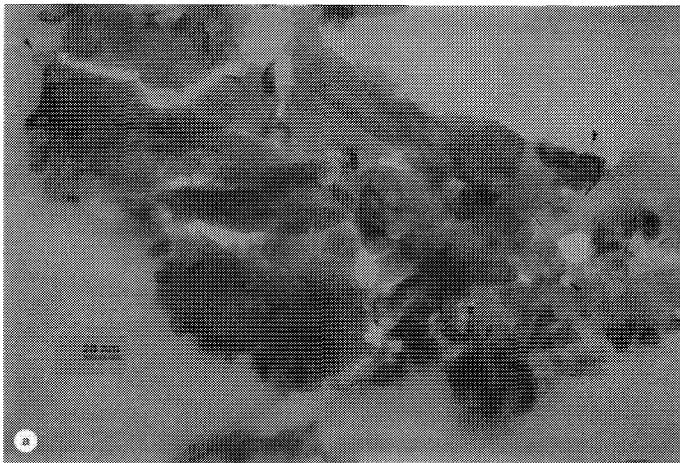
FIG. 7. TEM images of thin cuts in catalysts: (a) NiMo(10)S 1 Y-17 (sulfided at 593 K); (b) NiMo(10)S h Y-17 (sulfided at 673 K). Arrowheads show some MoS 2 microparticles.
